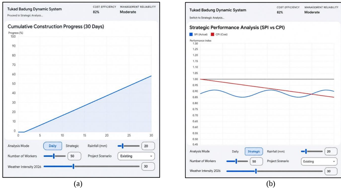
Figure 3. (a) Progress accumulation over representative 30-day peak rainfall window; (b) Performance indices (SPI vs CPI) under Baseline Scenario
