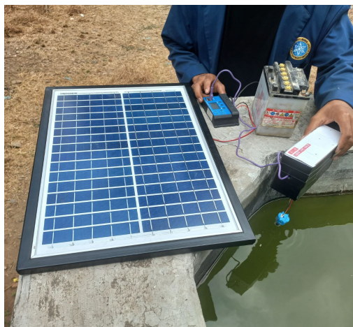
Gambar 5. Alat Monitoring Water Turbidity Berbasis PLTS
