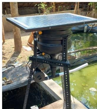
Gambar 6. Alat fish feeder
