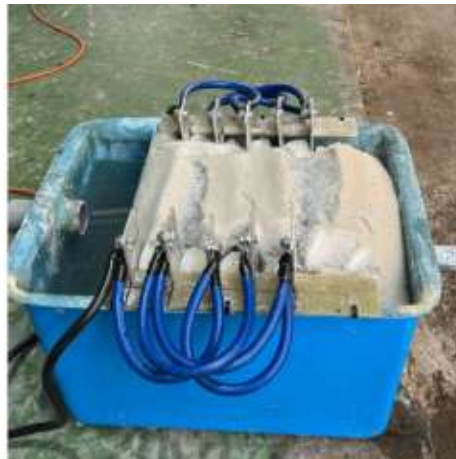
Figure 1. Electrocoagulation process using Al electrodes
