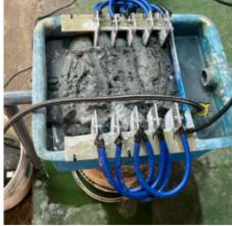
Figure 2. Electrocoagulation process using Fe electrodes
